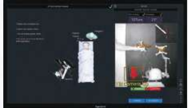
4. Set up: Position the tracker, calibrate new instruments and check their tip accuracy
